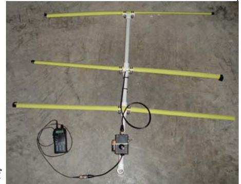
During the hunt, I realized that a little counter-weight needs to be added to this handle if you're going to be able to use the antenna comfortably for extended periods.
